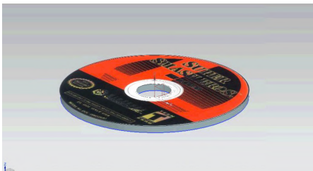
Disc. Functions most commonly used: extrude, extrude cut
